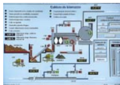
The heat plant is fully automated and this allows viewing and modifying any operative parameter in the facility from a central computer.
